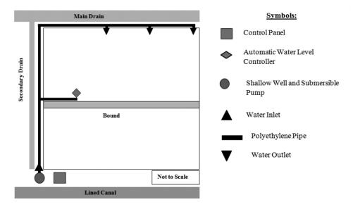
FIGURE 2. Schematic diagram of water distribution system at the study area
